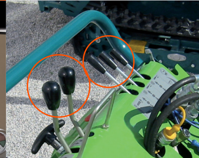
Application of I.222 and I.280 Duroplast handles
