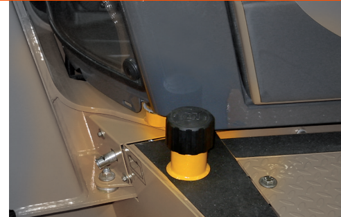
Application of SFV-VP double-valve pressurised breather cap "vandal-proof".
