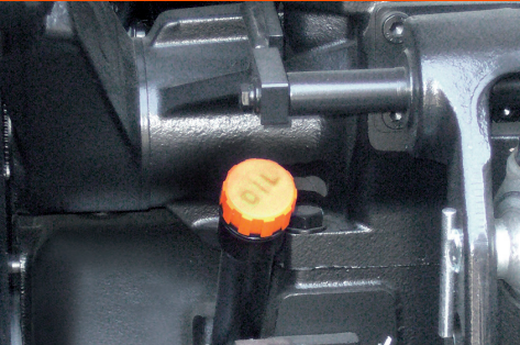
Application of SFP+a filler breather cap with splash guard and dipstick.
