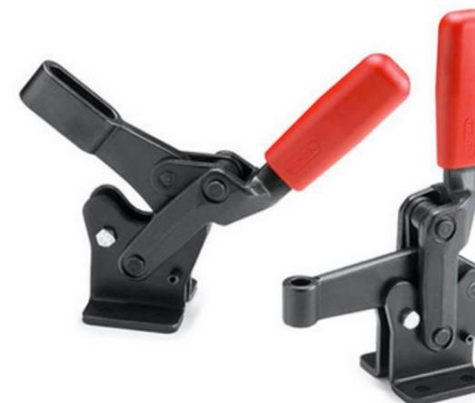
All the solutions guarantee perfect clamping with simple opening and closing motions, even in the presence of heavy shaking or vibrations: a special toggle-joint mechanism allows the clamping lever to reach an ample angle of rotation, while opening, with a slight movement of the components in order to vacate the working area
