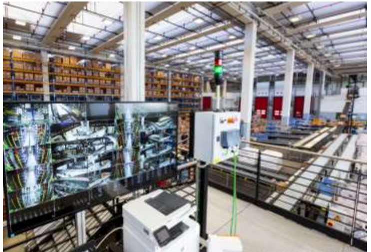
The Control Room with summary screens to which the images of the control cameras mounted on the individual shuttles are sent
