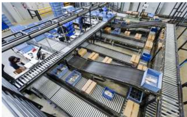
A glimpse at the picking stations with roller tracks coming from the automatic warehouse
