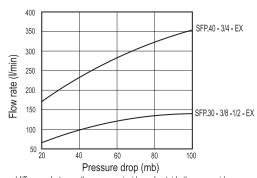
(difference between the pressure inside and outside the reservoir)
