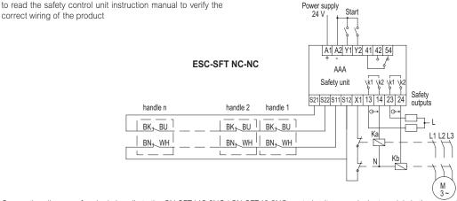
Connection diagram of a single handle to the CN-SFT.115-2NC / CN-SFT.46-2NC control units or equivalent models in the case of multiple handles with NC-NC contacts
