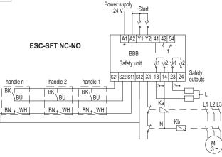
Connection diagram of a single handle to the CN-SFT.115-1NC+1NO / CN-SFT.46-1NC+1NO control units or equivalent models in the case of multiple handles with NC-NO contacts.
